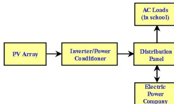
**Inverter** - The inverter changes the DC electricity produced by the modules into alternating current (AC) which is the type of electricity used in your school and homes.
