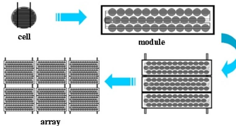
**Photovoltaic array** - The array which is made up of several photovoltaic modules converts or transforms sunlight directly into electric current. Like batteries, the current they produce is direct current (DC).
