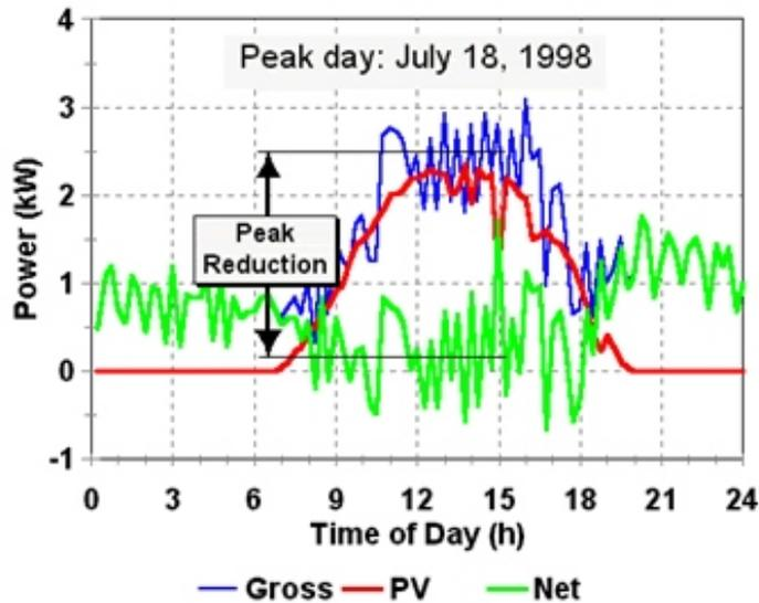
The interesting thing for Florida homeowners is the near match that the output from a photovoltaic array (red line) makes with the energy consumption of the house (blue line). When our houses are needing the most electricity for air conditioning, the systems are also producing the most power. If you're interested in more information about this study, the link to the zero home research and this particular one in Lakeland Florida is located in the Internet Sites section.
